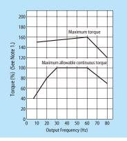
Note: 1. 100% of torque refers to the amount of torque that the motor produces when it is running at a 60Hz-synchronized speed. The starting torque is smaller in this case than that required when power is supplied from a commercial power line. So, the characteristics of the machine to be operated need to be taken into consideration.
