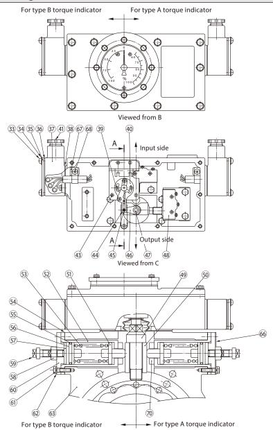
Figure 15-3 Torque Indicator
