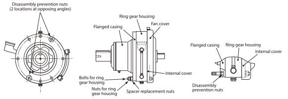
Figure 4-2 Construction Drawings
