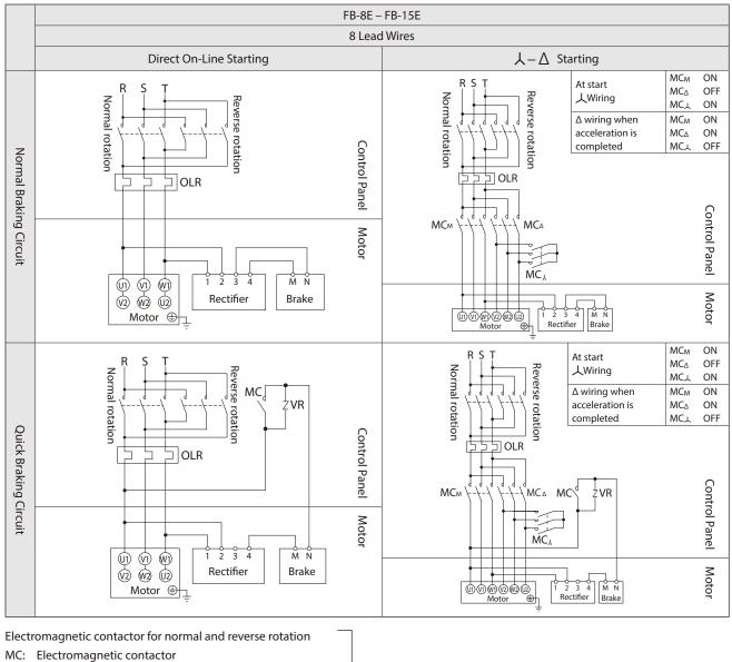
OLR: Overload protection device or electronic thermal relay
