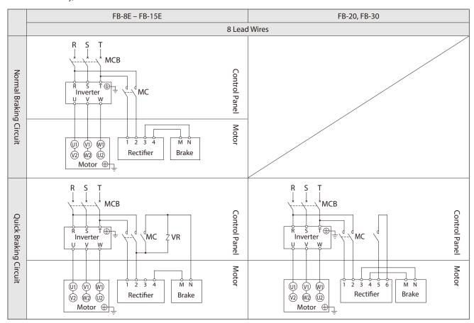
MC: Electromagnetic contactor
