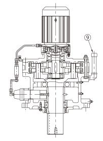
Figure 10-12 Type CVVM (Vertical, Gearmotor), 2 Stage Reduction (Example: Frame size 6225DA)
