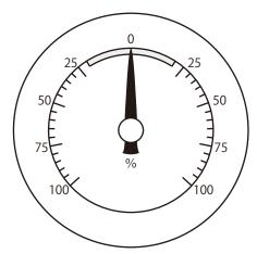
Figure 14-3 B-Type Torque Indicator (0 – 100% load factor display)
