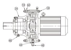
Figure 10-9 Type CHFM (Horizontal, Gearmotor), 1 Stage Reduction (Example: Frame size 6165)
