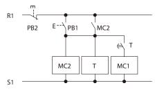
MC1: Electromagnetic contactor (Main motor)
