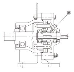
Figure 10-5 Type CNH (Horizontal, Reducer), 1 Stage Reduction (Example: Frame size 6105)
