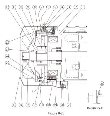
5 Brake release bolt 6 Spacer 7 Gap adjusting shims 8 Attachment bolt 9 Brake lining 10 Leaf spring 11 Boss 12 Shaft-retaining C-ring 13 Cover 14 Shaft-retaining C-ring 15 Fan 16 Fixed plate 17 Armature plate 18 Spring 19 Electromagnetic coil 20 Ball bearings 21 Motor shaft 22 Waterproof seal 23 V-ring 24 Waterproof cover attachment bolts 25 Waterproof cover 26 Shock absorber
