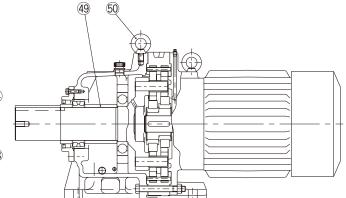
Figure 10-3 Type CHHM (Horizontal, Gearmotor), 1 Stage Reduction (Example: Frame size 6225)
