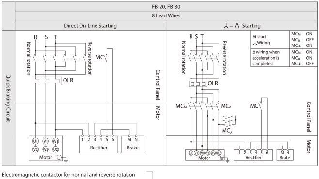
MC: Electromagnetic contactor
