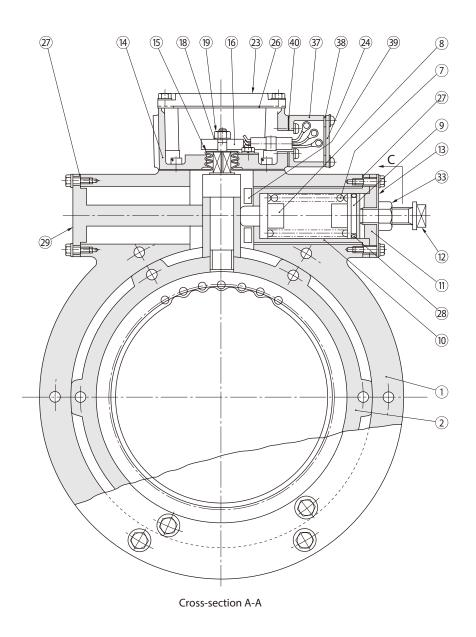
Figure 15-2 Type CHHM (Horizontal, Gearmotor), 3 Stage Reduction
