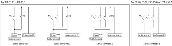
Note : For inverter drives, connect to the R phase (power source side).
