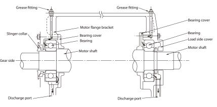
Gear Side Bearing Construction
