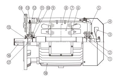
Figure 10-21 Direct-coupled motor for CYCLO Drive (Open bearing structure) (Example: N-200LS 30kW 6P)
