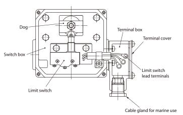
Figure 11-2 Terminal Box-Switch Box
