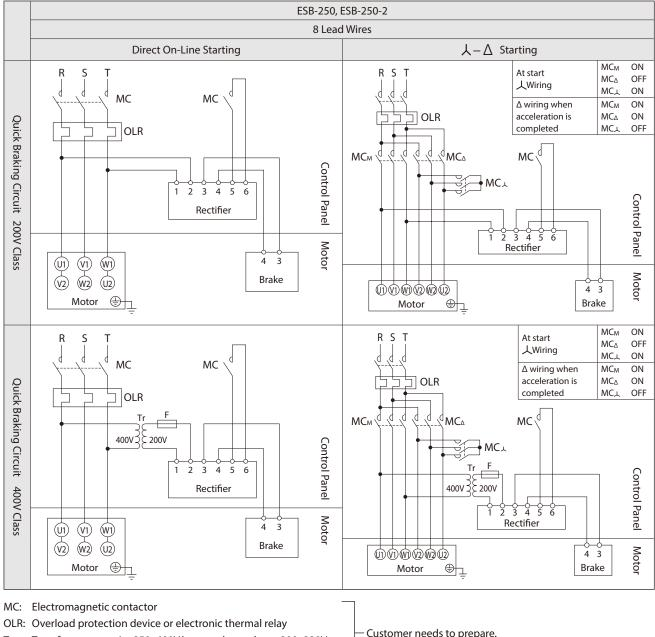
Transformer capacity 250–600VA, secondary voltage 200–220V Tr:
