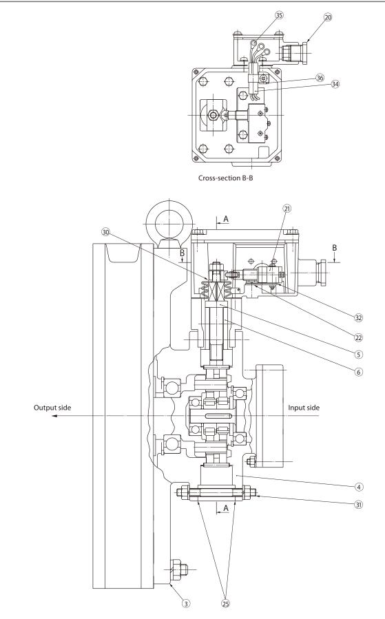
Figure 15-1 Type CHHM (Horizontal, Gearmotor), 3 Stage Reduction
