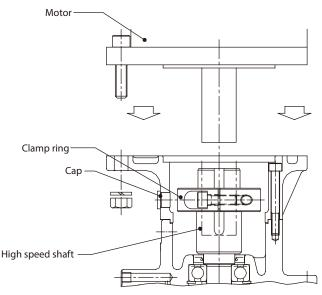
Figure 4-2 Assembly Diagram
