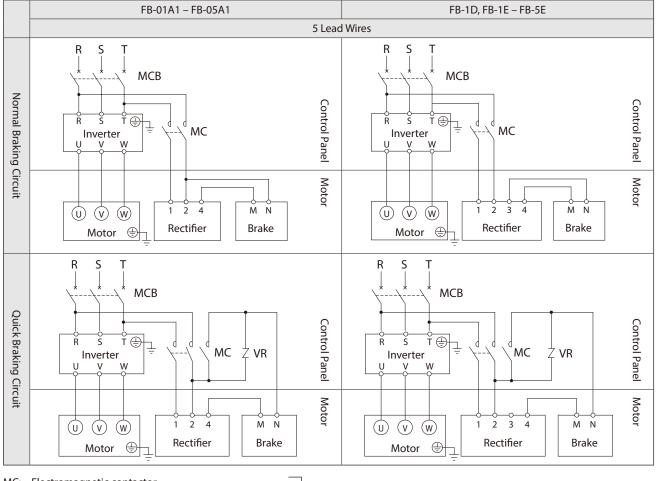
MC: Electromagnetic contactor
