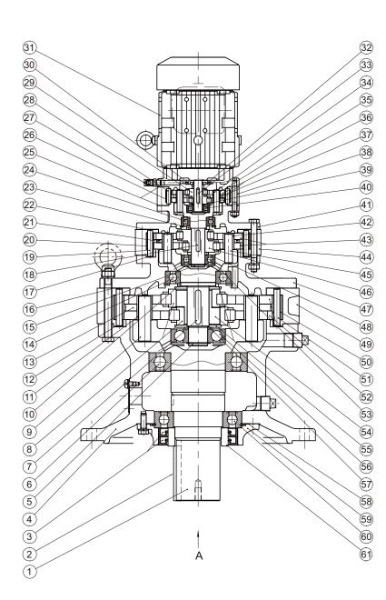
Figure 10-13 Type CVVM (Vertical, Gearmotor), 3 Stage Reduction (Example: Frame size 6185TD)
