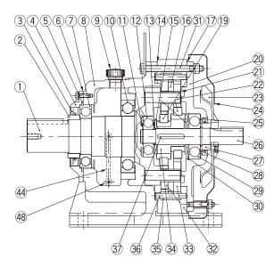
Figure 10-1 Type CHH (Horizontal, Reducer), 1 Stage Reduction (Example: Frame size 6175)
