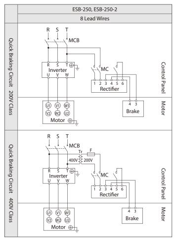
MC: Electromagnetic contactor
