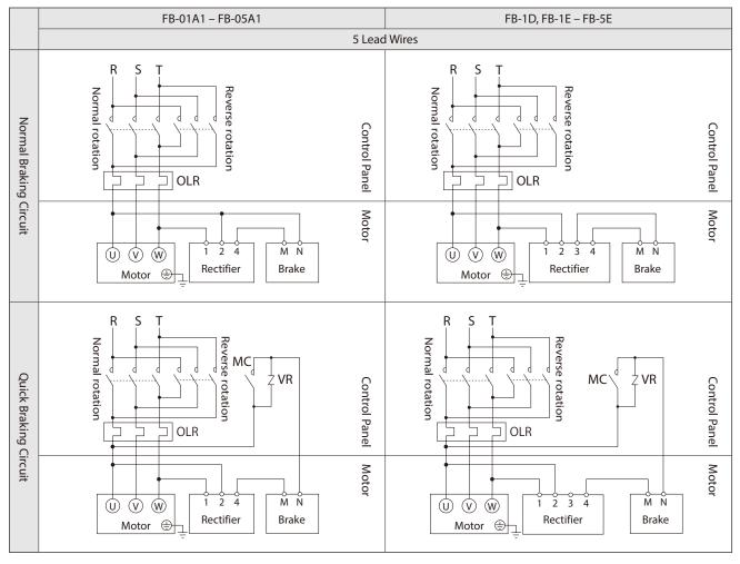
Electromagnetic contactor for normal and reverse rotation
