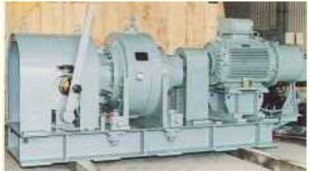
Inching Device for Cement Mill
