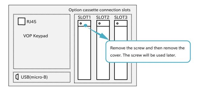
(2) Attach the P1-PB. The slots 2 and 3 have one more connection in the lower side. However, the P1-PB will not need that connection.
