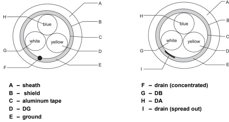
Figure 14 Cable Diagram
