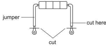
Figure 15 Terminal Resistor
