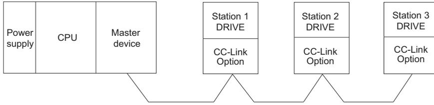
Figure 18 Connecting Multiple Drives on the Same Network
