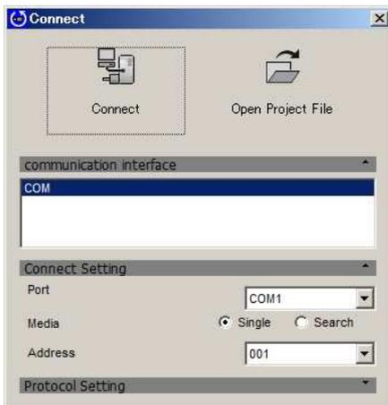
If SDWP001 is unable to communicate with the drive, the window above will not appear and the following message will be displayed instead:
