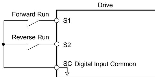
Figure 4.13 Example Wiring Diagram for 2-Wire Sequence
