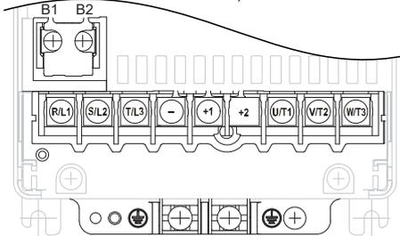
Figure 3.3 Main Circuit Terminal Block Configurations
