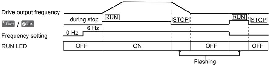
Figure 4.2 RUN LED and Drive Operation
