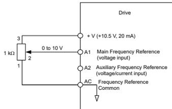
Figure 4.11 Voltage Input for the Main Frequency Reference
