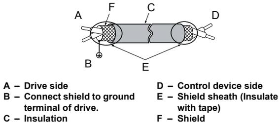
Figure 3.18 Preparing the Ends of Shielded Cables
