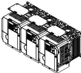
Figure 2.4 IP20/NEMA Type 1 Side-by-Side Mounting in Enclosure
