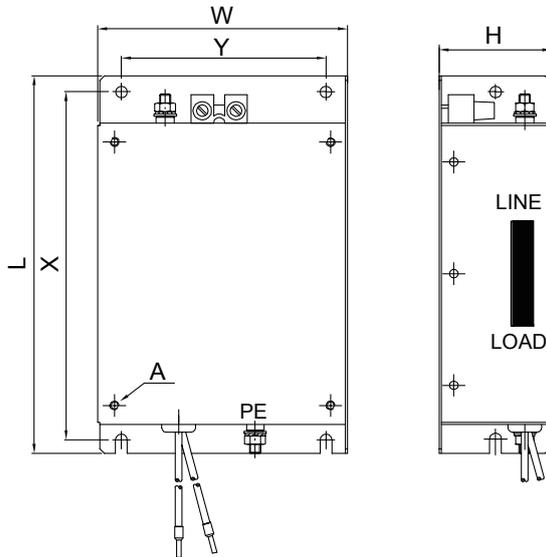
Figure C.5 EMC Filter Dimensions
