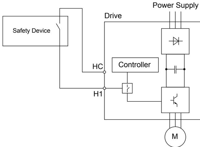
Figure C.10 Safe Disable Wiring Example
