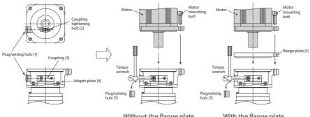
Without the flange plate for a motor
