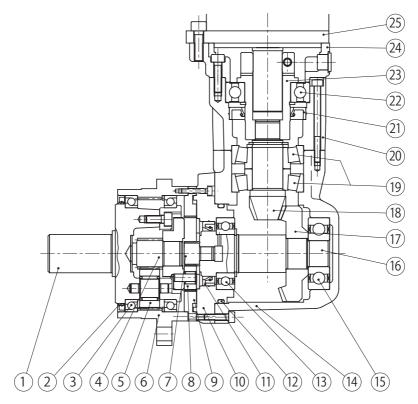
Figure 10-2 PK1 Type Triple-reduction (example: ANFX-PK120N)
