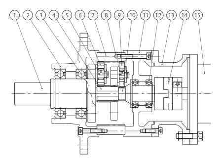
Figure 10-5 L Type Double-reduction (example: ANFJ-L40)
