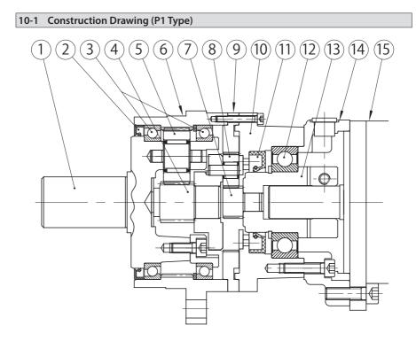
Figure 10-1 P1 Type Double-reduction (example: ANFX-P120N)
