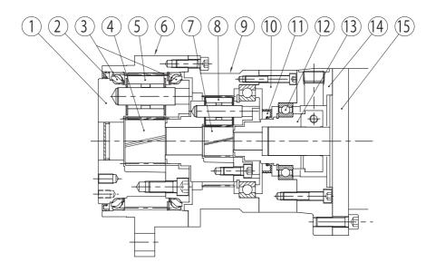
Figure 10-3 P2 Type Double-reduction (example: ANFX-P250F)
